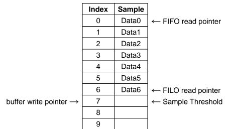
Figure 21: Buffer Approaching Sample Threshold
