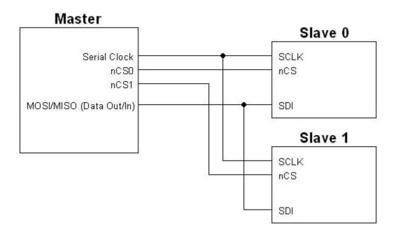
Figure 7: 3-wire SPI Connections
