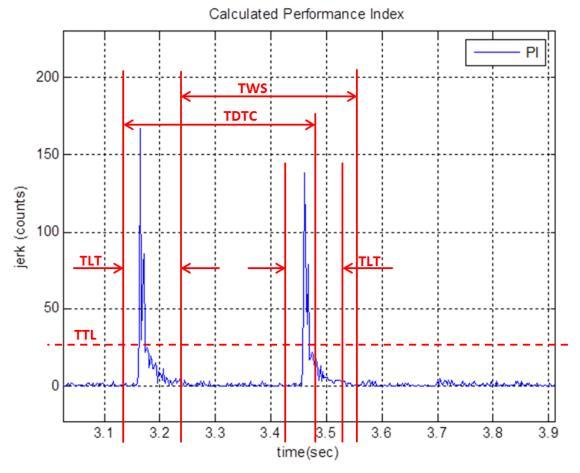
Figure 16: Double-Tap<sup>™</sup> Timing
