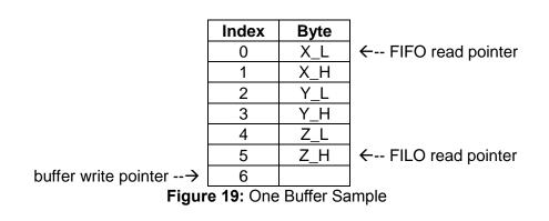
Regardless of the selected mode, the buffer fills sequentially, one sample at a time. Note in Figure 20 the location of the FILO read pointer versus that of the FIFO read pointer. The buffer write pointer shows where the next sample will be written to the buffer.
