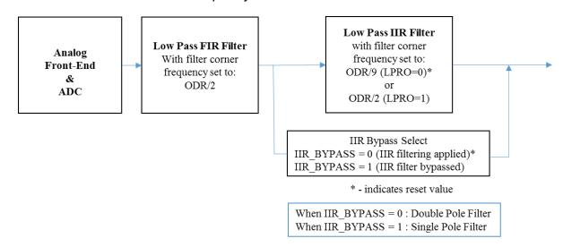
Figure 10: Low-Pass Filter Design and Control Circuitry
