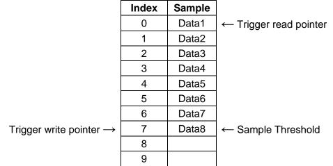
Figure 23: Additional Data Prior to Trigger Event
