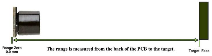
In general, the HRLV-MaxSonar-EZ will report the range to the leading edge of the closest detectable object. Target detection has been characterized in the sensor beam patterns.
