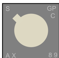
Figure 9 Laser marking on SGPC3. The pin-1 location is indicated by the keyhole pattern in the light-colored central area. The bottom line contains a 4-digit alphanumeric tracking code
